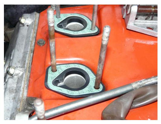
19. Pictures of new manifolds with injector bores.
