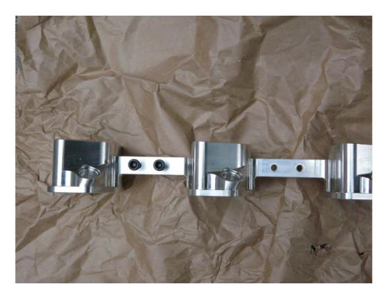
20. Install injector blocks over gasket/spacer stack on intakes.
