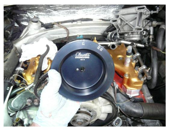
33. The new trigger mount is held in by the bolt formerly used to hold the distributor down. Install the motor mount and verify that the sensor holder seats properly on the engine block. It may be necessary to grind away some material to clear the sensor mount.
