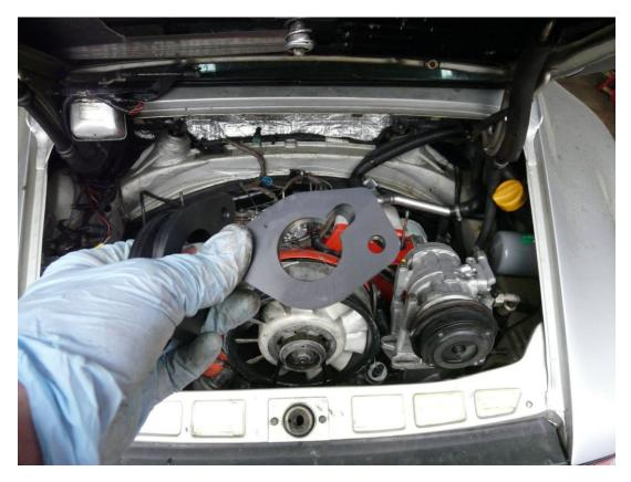
16. Install six 3.2 Carrera intake gaskets.
