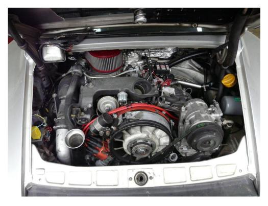
11. After you have removed all the intake and CIS components, etc. plug all intakes and turbo pipes with towels to prevent dirt or parts from falling into them.
