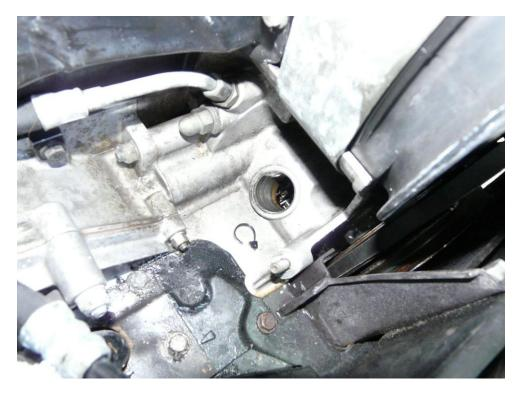
29. Insert your Clewett distributor hole plug and tighten it with a 8mm allen wrench.
