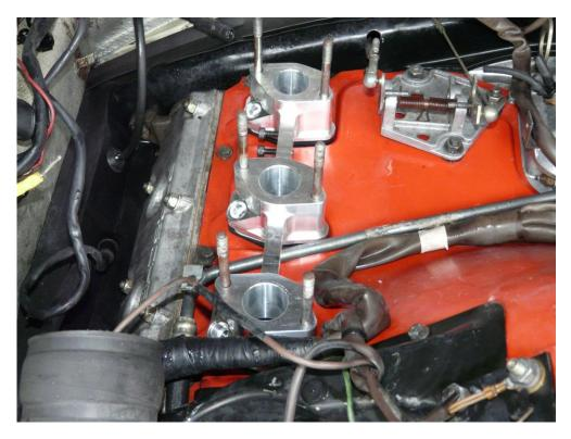
21. Install six 930 gaskets over top of intake blocks.
