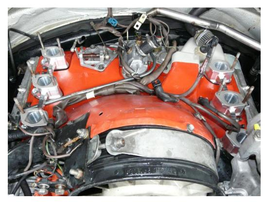
23. Install manifold on top of gaskets and blocks.
